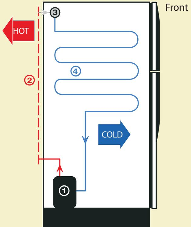
river with a hole in the dam. The water leaking through the hole is at a low pressure on the downstream side; the water on the other side (being held back by the dam) is at a high pressure. Once again, the pressure/temperature relationship (lower pressure/lower temperature) creates a cold, low pressure liquid refrigerant that gets fed to the evaporator (4).
